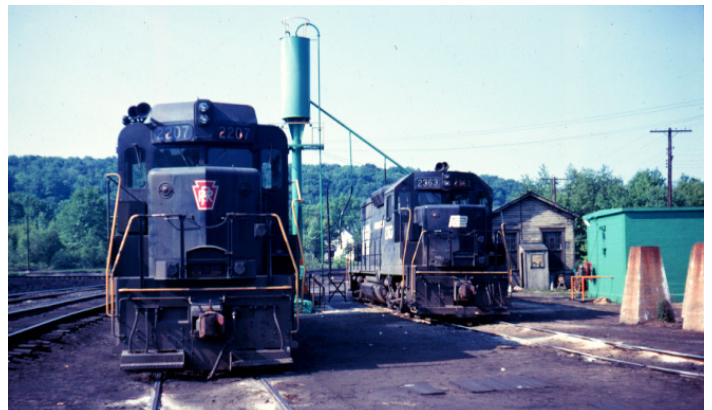
The sand tower is visible behind the two diesel locomotives. The first building to the right was the oil house with the car repair shop located directly behind.
